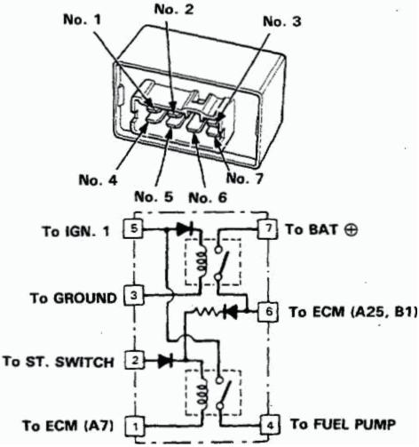
3. Attach the battery positive terminal to the No. 5 terminal and the battery negative terminal to the No. 3 terminal of the PGM-FI main relay. Then check that there is continuity between the No. 7 terminal and No.6 terminal of the PGM-FI main relay.
